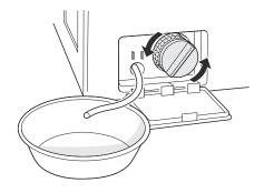
**5** Clean the pump filter and opening.
