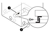
3 Preassemble a 4" (10 cm) elbow ⑤ to the next 4" (10 cm) duct section, and secure all joints with duct tape. Be sure that the male end of the elbow faces AWAY from the dryer. Insert the elbow/duct assembly through the side opening and press it onto the adapter duct. Secure it in place with duct tape. Be sure that the male end of the duct protrudes 1 1/2" (3.8 cm) to connect the remaining ductwork. Attach the cover plate ⑥ to the back of the dryer with the included screw.
