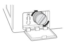
**8** Close the drain pump filter cover.
