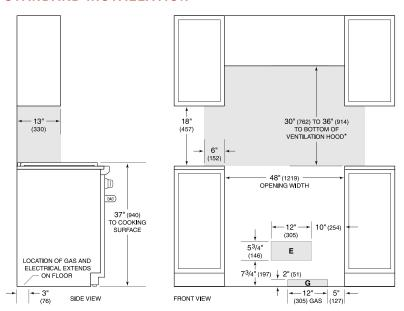
\*Without ventilation hood, 42\*(1067) minimum clearance countertop to combustible materials, charbroiler and GR488 require non-combustible materials. NOTE: Shaded area above countertop indicates minimum clearance to combustible surfaces,
