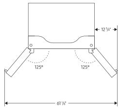
NOTE: Please allow 33/4" of clearance when installing along a wall
