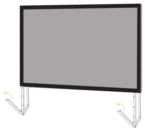
**11.** Connect the front support brace to the front piece of the screen leg using two (2) hand screws so the projection screen is stable. Then, do the same for the second front support brace.
