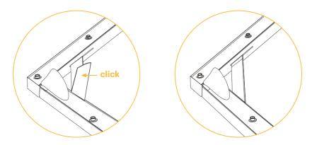
**3.** Then, take out the screen fabric and place it at one corner of the frame. Next, start unfolding the fabric until it is completely spread out within the frame.
