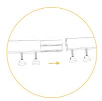
**8.** Align the holes of the screen legs with the holes on the screen frame. Then, fasten the screen legs to the frame using three (3) hand screws for each leg.
