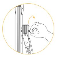
**7.** Lay the frame on a flat surface with the screen frame facing up and place the screen legs on back of the frame.
