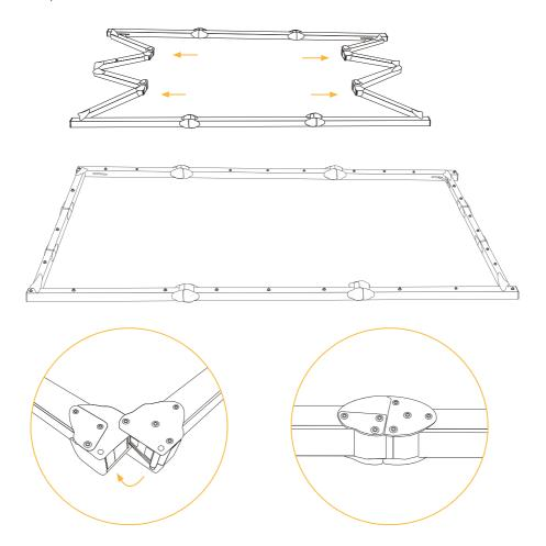
**NOTE:** You should hear a click sound to know when joints of the frame are securely locked in place.
