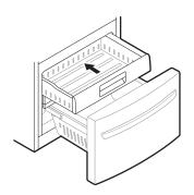
Replace the ice bin in the drawer. Insert the Durabase basket in the rail assembly.
