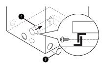
Preassemble a 4" (10 cm) elbow 5 to the next 4" (10 cm) duct section, and secure all joints with duct tape. Be sure that the male end of the elbow faces AWAY from the dryer. Insert the elbow/duct assembly through the side opening and press it onto the adapter duct. Secure it in place with duct tape. Be sure that the male end of the duct protrudes 1 1/2" (3.8 cm) to connect the remaining ductwork. Attach the cover plate 6 to the back of the dryer with the included screw.
