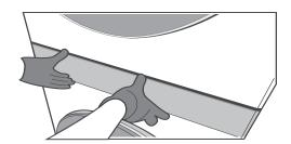
5 Disconnect the wire harnesses from the washer **1** and dryer **2** to the control panel.
