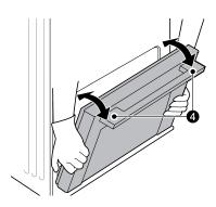
Lift and pull the door towards you until the hinge latches are completely loosened.
