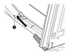
Slowly open the door fully. Make sure that the hinges **2** are properly engaged in the slots ❸.
