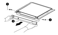
Wearing safety gloves, grab and lift the glass panel 3 slightly with both hands and pull it forward to remove it from the oven door. Set the glass aside on a protected surface. Set aside the gaskets (4 ea) inserted into the
