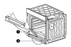
2 Fully insert the hinges 2 into the slots 3.
