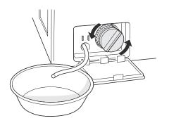
**5** Clean the pump filter and opening.
