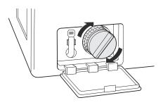
**8** Close the drain pump filter cover.
