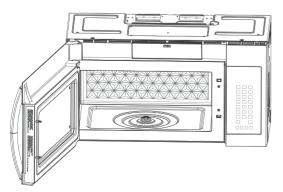
• Remove the charcoal filter by pushing the top of the filter inwards, then pull it forward out from the unit.
