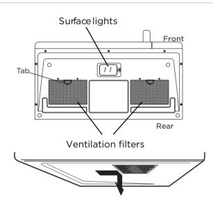
• To remove the exhaust ventilation filters, slide the filter to the rear. Then pull filter downward and push to the other side. The filter will drop out. Repeat for the 2nd filter.
