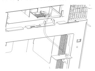
• Re-install LED light to the bracket with mounting screw.
