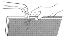
• Soak the ventilation filters in hot water using a mild detergent. Rinse well and shake to dry or wash in a dishwasher. Do not use ammonia. The aluminum on the filter will corrode and darken.
