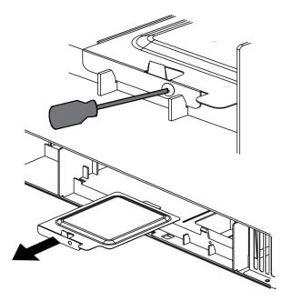
Remove the LED bracket and light assembly. Remove the LED light from the bracket by removing the mounting screw and replace only with part 5304499540. To order parts call 800-599-7569.
