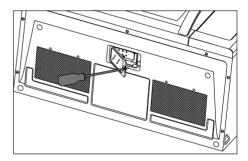
• Remove the LED light mounting screw.
