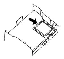
• Replace the charcoal filter (if installed). Push the vent grill back into place (engaging both the bottom and top tabs) and replace the vent grill mounting screws. SERVICE CALL CHECK 23
