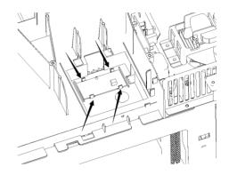
• Replace the microwave oven light cover by carefully pushing into place (make sure the light cover rear tab is inserted into slot at rear), replace the screw.
