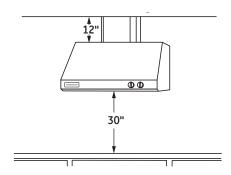
8 FT. CEILINGS When the hood is installed 30" above the cooking surface and there is no soffit or upper cabinetry, order one 12" duct cover accessory.
