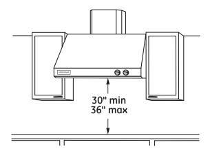
For this installation, a decorative duct cover is available to conceal the ductwork running from the top of the hood. Use of the duct cover requires special consideration to the installation height above the countertop.
