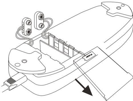
**Step 2.** Install two 9V batteries alkaline (Model# 6LR61) in the external transformer (fig. 1.1).
