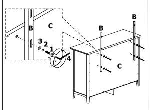
\*DO NOT FULLY TIGHTEN BOLTS UNTIL FINAL STEP.
