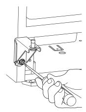
7. Relocate plastic spacer/bushing on top and bottom of door to opposite side. Clean out bushing hole in door bottom with a screwdriver if necessary.
