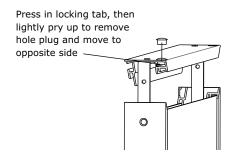
11. Place door on lower hinge pin. Invert and install upper hinge on door. Fasten upper hinge to unit (three screws). Partially tighten screws.
