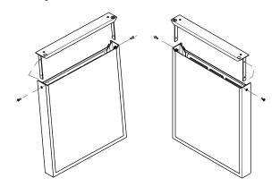
9. Remove plastic hole plug from door handle and relocate to opposite side. Lift the handle slightly and press on the locking tab, then gently pry the hole plug out of the hole, being careful not scratch the top cap.
