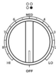
The control knobs can be set to anywhere between HI and LO. Push in and turn to setting.
