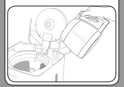
Insert the permanent gold tone filter or paper filter into the filter basket holder.
