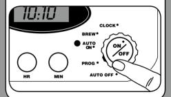
To program the Auto Off: Turn the Function Knob to Auto Off. Use the Hour and Minute buttons as in #1 (to set the time) to program your coffeemaker to shut off from 0 to 4 hours after brew cycle is finished.
