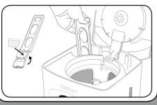
Pour desired amount of water into the water reservoir. A water level indicator is located on the side of the unit.
