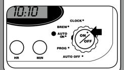
To start the brew cycle at the same time the next day, simply press the On/Off button and release. The green indicator light will illuminate.
