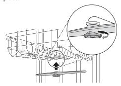
7 After assembly, make sure that the spray arms rotate freely.
