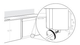
Use a Phillips screwdriver to remove 2 screws
