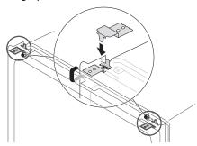
**2** Bend the tabs on the brackets to secure them to the frame using a pair of needle nose pliers.
