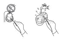
To reassemble the vent cover, place it over the supply tube in the same orientation as it was removed (about 2 o'clock). Turn the cover counterclockwise until it clicks into place.
