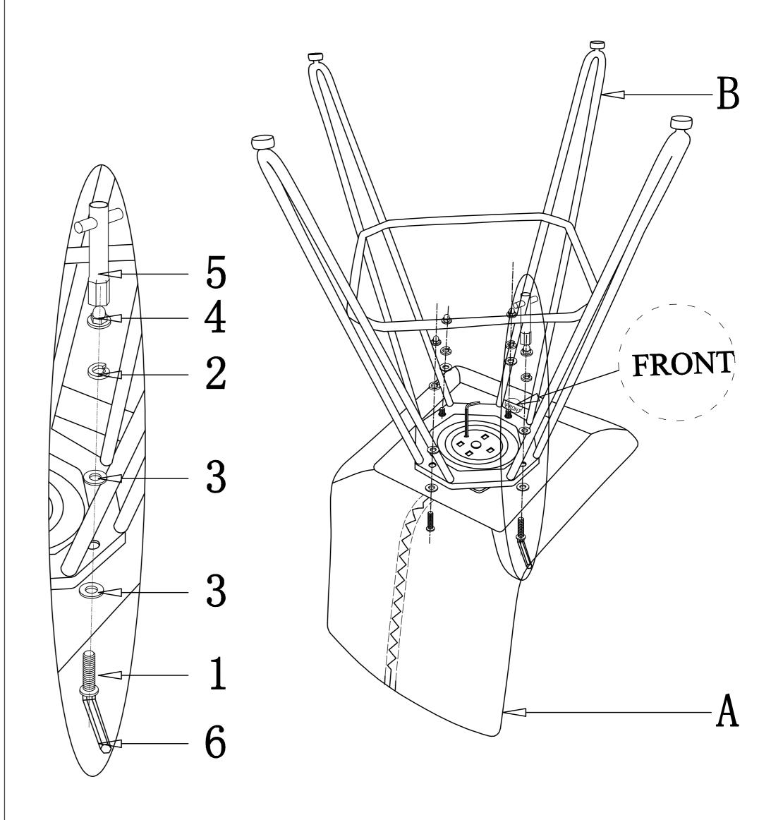
STEP 3. WHEN ALL BOLTS ARE COMPLETELY TIGHTENED, REMOVE THE ALLEN KEY FROM THE SWIVEL MECHANISM AND FLIP THE CHAIR RIGHTSIDE UP.
