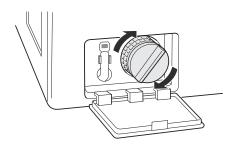
Close the drain pump filter cover.
