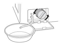
Clean the pump filter and opening.
