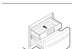
Replace the ice bin in the drawer. Insert the Durabase basket in the rail assembly.
