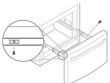
Insert the drawer into the frame, and push the drawer back until it clicks into place.
