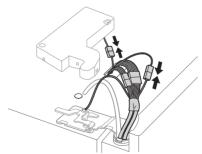
Push the water supply tube into the hole on the top case and pull it through the backplate.
