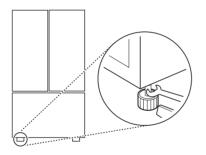
Open both doors and check to make sure that they close easily. If the doors do not close easily, tilt the refrigerator slightly more to the rear by turning both leveling legs to the left. It may take several more turns, and be sure to turn both leveling legs the same amount.
