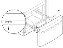
Grip both sides of the drawer and pull it up to remove it from the rails.
