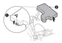
Detach all the wire harnesses 3. Unscrew the ground wire **4**. Remove the cover.
