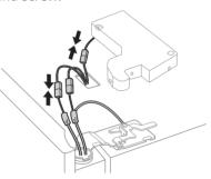
Set the hinge cover 4 in place. Insert and tighten the cover screw **5**.
