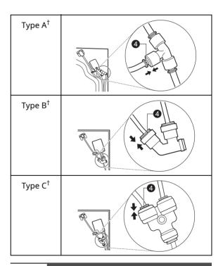
· Disassembling/Assembling the Water Lines
