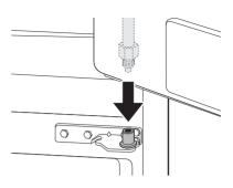
Fit the hinge 1 over the hinge lever latch 2 and slot it into place. Rotate the lever 3 counterclockwise to secure the hinge.
