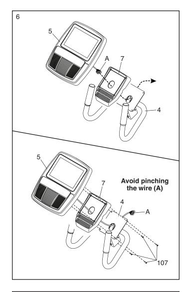
7. While a second person holds the Console Bracket (4) near the Frame (1), connect the wire (A) on the Console (5) to the Main Wire (115). Tip: The wire connectors should slide together easily and snap into place with an audible click. If they do not, turn one connector and try again.
