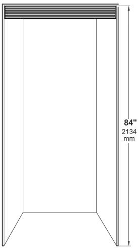
The cabinet opening height is 84" when using the decorative grille. The decorative grille is deliverable as accessory and is not required for proper operation of the appliance. All ventilation requirements are handled through the toe kick grille on the appliance and this decorative grille is intended to be used as a filler for pre-existing 84" openings.
