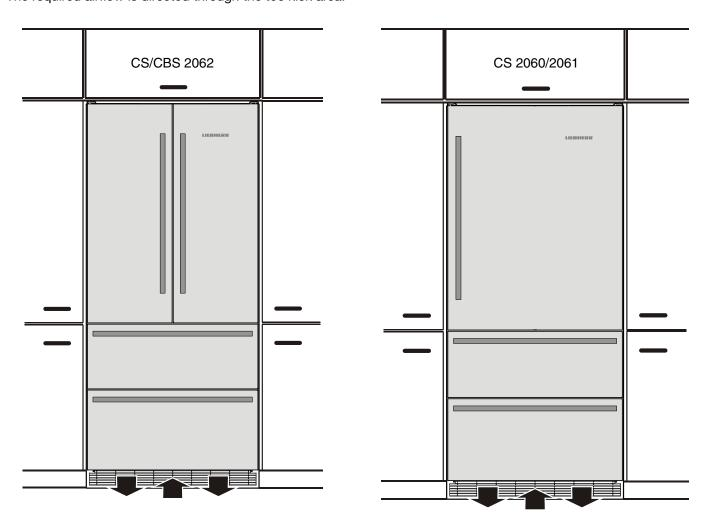
It is important to use the provided cover grille for the ventilation opening. This opening must not be covered.
