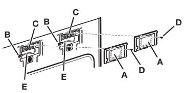
Before you start, disconnect power. Remove hold-down screw (D) and terminal block cover (A).
