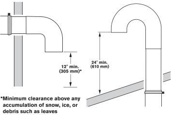
If the main vent travels vertically through the roof, rather than through the wall, install a 180° sweep elbow on the end of the vent at least 2 ft. (610 mm) above the surface of the roof.
