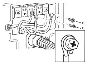
**3.** Connect remaining wires under outer terminal block. Tighten screws.
