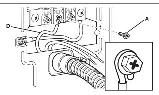
**3.** Place hooked ends of remaining direct wire cables (hooks facing right). Squeeze hooded ends together and tighten screws. Finally, re-install terminal block cover and tighten hold-down screw. Tighten screws. Go to "Complete Installation" section.
