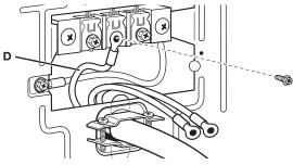
2. Connect remaining wires with outer terminal block screws (F). Tighten screws. Finally, re-install terminal block cover and tighten hold-down screw. Go to "Complete Installation" section.
