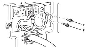
4. Connect a separate copper ground wire (G) under the external ground conductor to screw (C) an adequate ground. Finally, re-install terminal block cover and tighten hold-down screw. Go to "Complete Installation" section.
