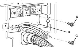
Connect neutral ground (B) and place hooked end (hook facing right) of neutral wire (white or center wire) cable under center terminal block screw (B). Squeeze hooked end together. Tighten screw.
