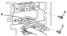
2. Connect neutral ground wire (B) and neutral wire (white or center) (D) of power supply cord/cable under center terminal block. Tighten screw.
