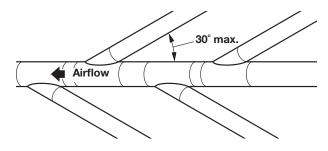
The maximum angle of each vent entering the main vent should be no more than 30°.
