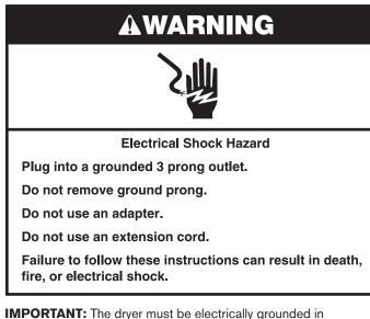
**IMPORTANT:** The dryer must be electrically grounded in accordance with local codes and ordinances or, in the absence of local codes, with the National Electrical Code, ANSI/NFPA 70, latest edition, or Canadian Electrical Code, CSA C22.1. If codes permit and a separate ground wire is used, it is recommended that a qualified electrical installer determine that the ground path is adequate.
