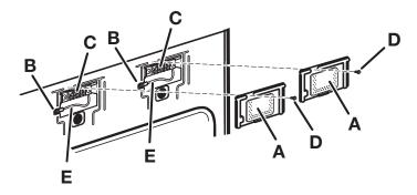
Before you start, disconnect power. Remove hold-down screw (D) and terminal block cover (A).
