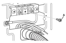
Place hooked end (hook facing right) of neutral wire (white or center wire) (D) cable under center terminal block screw (B). Squeeze hooked end together. Tighten screw.
